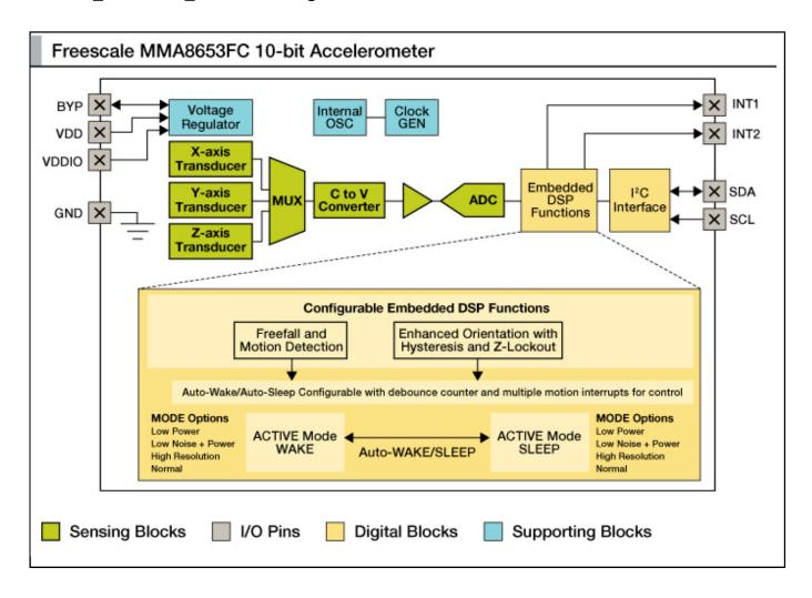
View additional information for ±2g/±4g/±8g, Low g, 10-Bit Digital Accelerometer.
