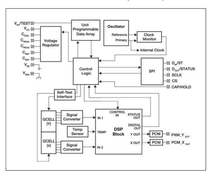
View additional information for SPI ±3.5 g or ±5.0 g XY-Axis, Low-g, Digital Inertial Sensor.
