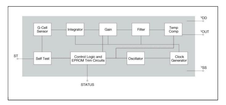
View additional information for ± 7g, Low-g, Analog Accelerometer.
