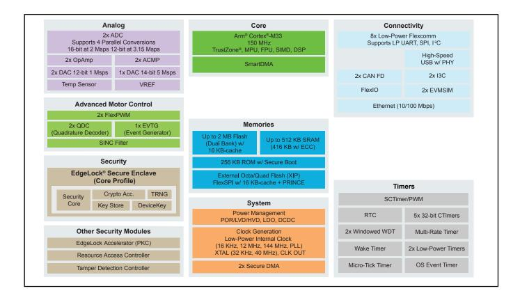
View additional information for MCX N94, N54, N53, N52 and N24 with Highly Integrated Low-power Dual Core Arm® Cortex®-M33 MCUs, with on-chip Accelerators and Advanced Security.
