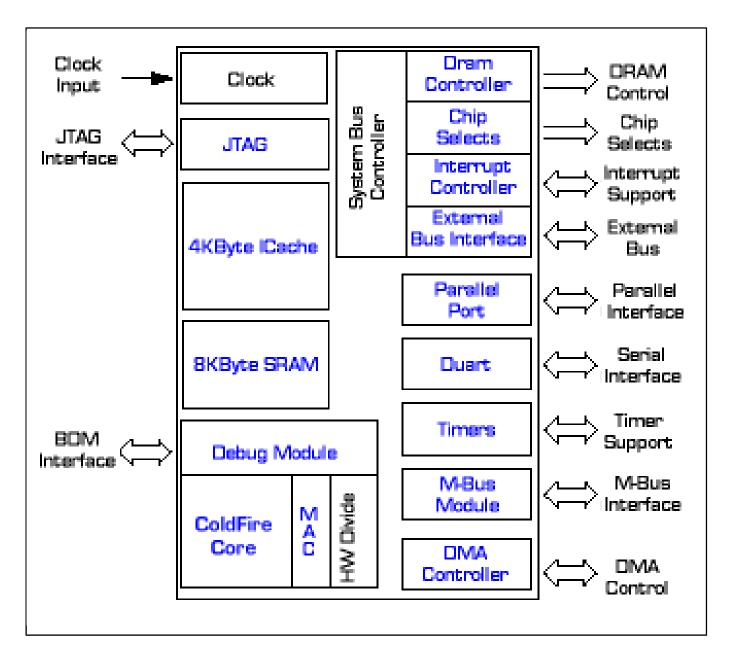
View additional information for Integrated ColdFire® Microprocessor with DMA.
