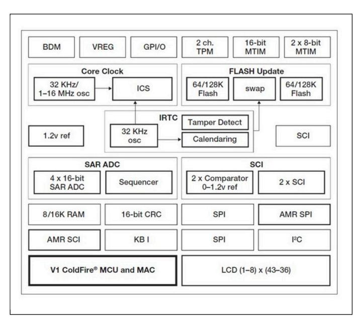
View additional information for MCF51EM256 32-Bit MCU for Smart Meter Applications.
