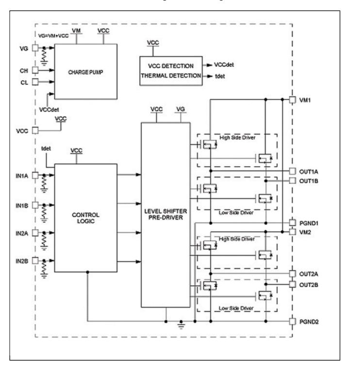
View additional information for H-Bridge Motor Driver, 2-7 V, 1.4 A, 200 kHz.
