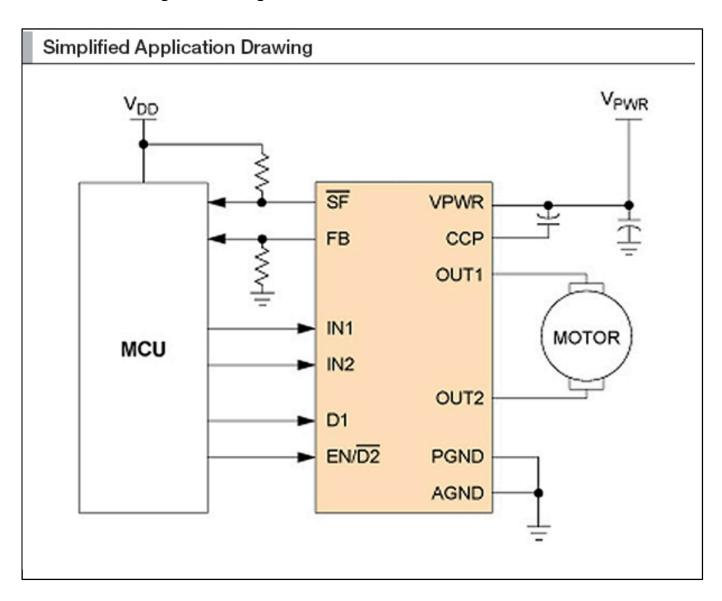
View additional information for MC34931/S H-Bridge, Brushed DC Motor Driver, 5-36 V, 5 A, 11 kHz/20 kHz.
