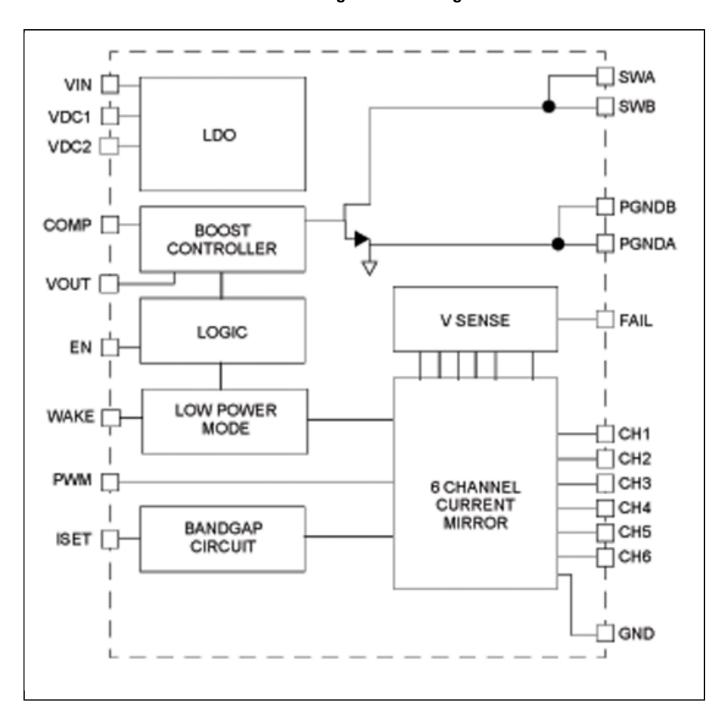
View additional information for 6 Channel LED Backlight Driver with Power Supply.
