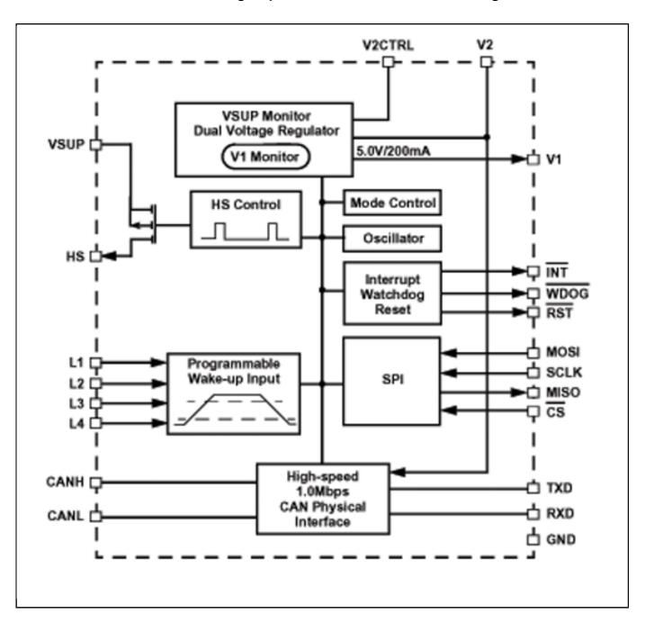
View additional information for SBC with Enhanced High-Speed CAN Transceiver.
