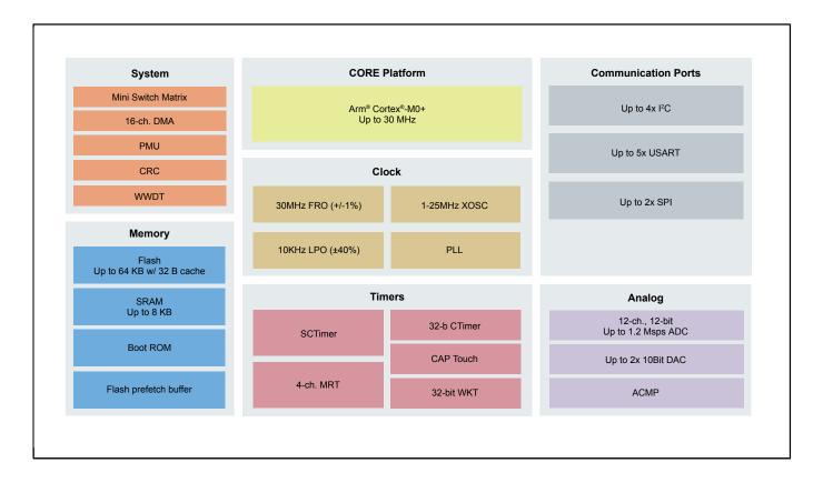
View additional information for LPC840: 32-Bit Arm® Cortex®-M0+-Based Low-Cost MCU.
