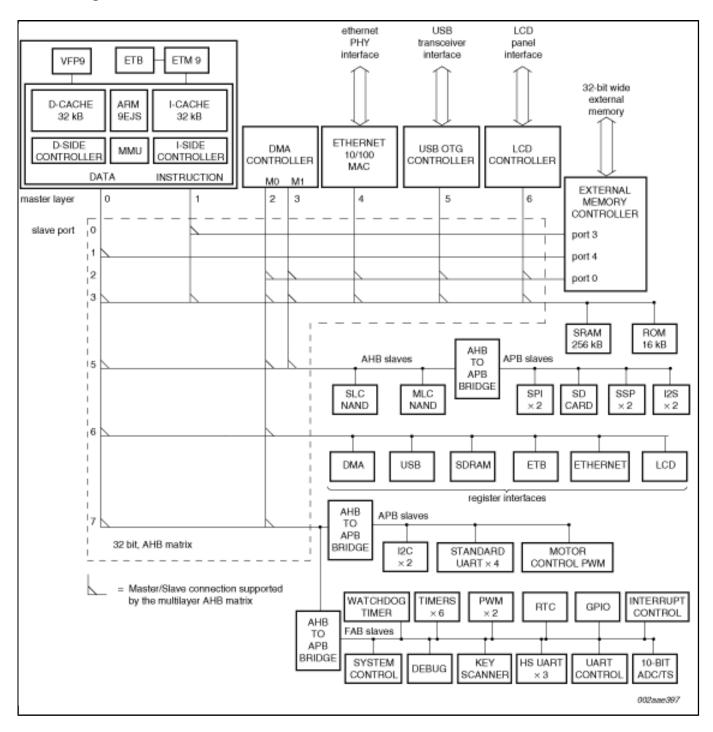
View additional information for Arm926EJ-S™ with 256 kB SRAM, USB High-speed OTG, SD/MMC, NAND flash controller, Ethernet.
