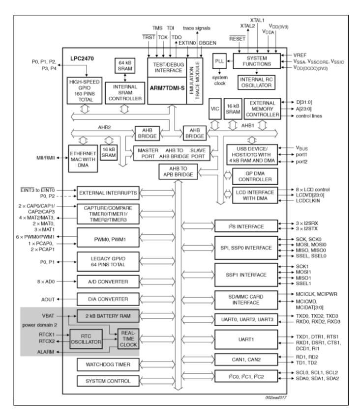
View additional information for Flashless 16-bit/32-bit microcontroller; Ethernet, CAN, LCD, USB 2.0 device/host/OTG, external memory interface.
