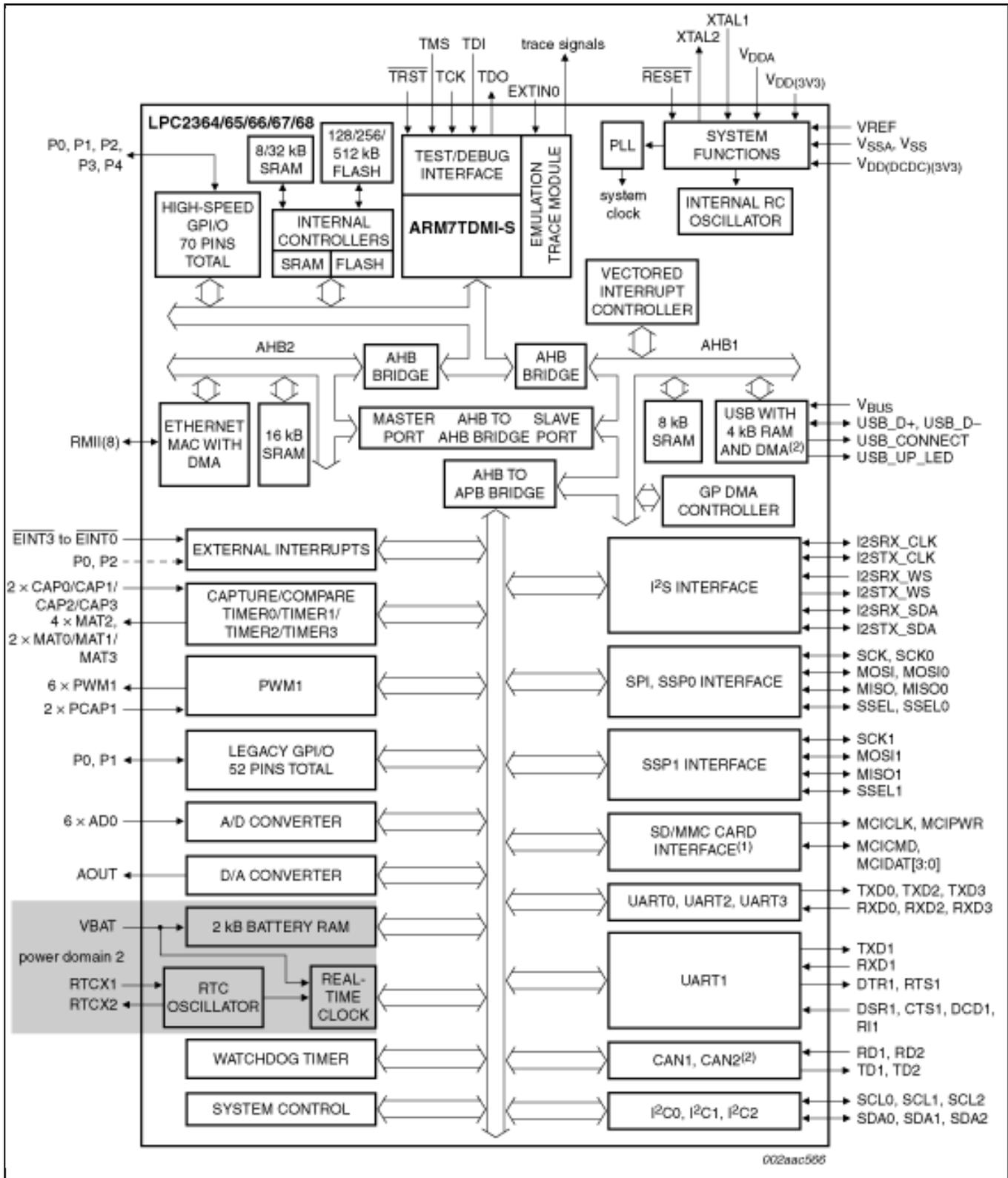
View additional information for [Arm7™ with 512 kB flash, 58 kB SRAM, Ethernet, USB 2.0 Device, CAN, SD/MMC, and 10-bit ADC.](#)
