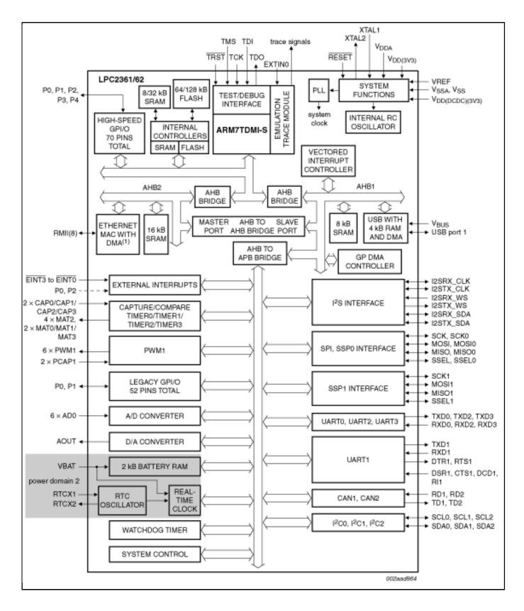
View additional information for Single-chip 16-bit/32-bit MCU; up to 128 kB flash with ISP/IAP, Ethernet, USB 2.0 device/host/OTG, CAN, and 10-bit ADC/DAC.
