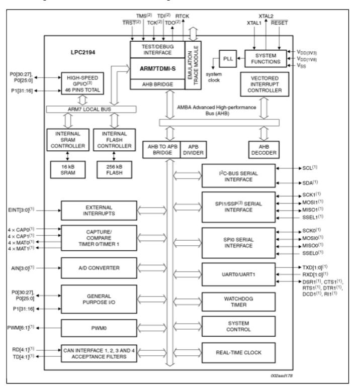
View additional information for Single-chip 16/32-bit microcontroller; 256 kB ISP/IAP flash with 10-bit ADC and CAN.
