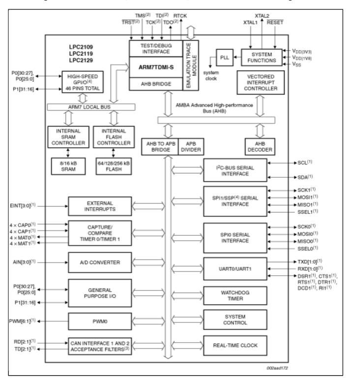
View additional information for Single-chip 16/32-bit microcontrollers; 64/128/256 kB ISP/IAP flash with 10-bit ADC and CAN.
