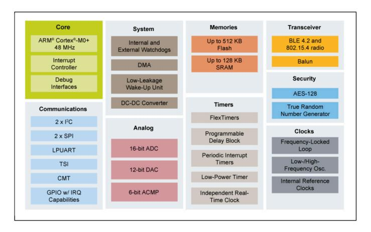
View additional information for Kinetis® KW41Z-2.4 GHz Dual Mode: Bluetooth® Low Energy and 802.15.4 Wireless Radio Microcontroller (MCU) based on Arm® Cortex®-M0+ Core.
