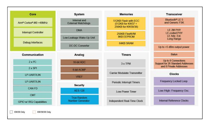
View additional information for KW39/38/37: 32-Bit Bluetooth 5.0 Long-Range MCUs with CAN FD and LIN Bus Options, Arm® Cortex®-M0+ Core.
