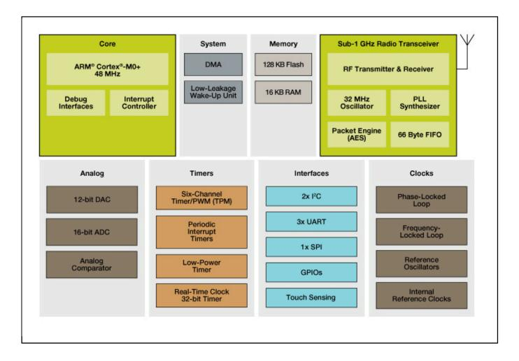
View additional information for Kinetis® KW0x-48 MHz, Sub-1 GHz Wireless Radio Microcontrollers (MCUs) based on Arm® Cortex®-M0+ Core.
