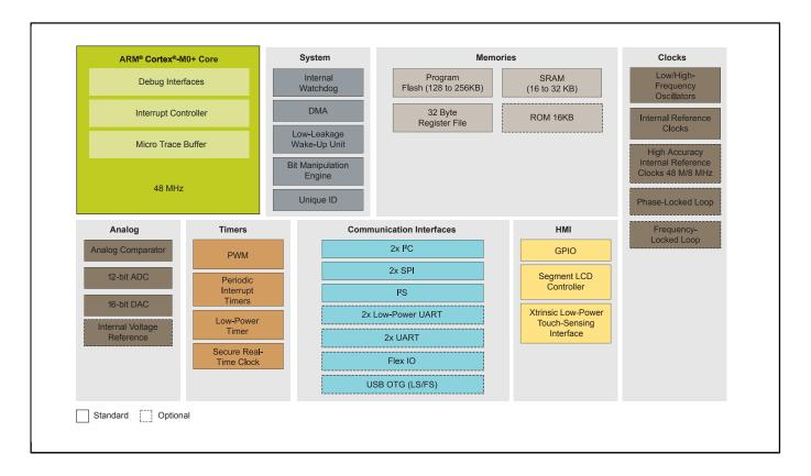
View additional information for Kinetis® KL4x-48 MHz, USB, Segment LCD, Ultra-Low-Power Microcontrollers (MCUs) based on Arm® Cortex®-M0+ Core.
