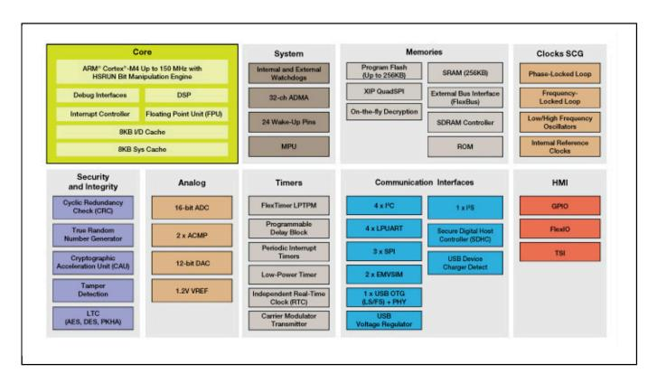
View additional information for Kinetis K81-150 MHz HW Cryptographic Co-Processor, Anti-Tamper and QuadSPI Microcontrollers (MCUs) Based on Arm® Cortex®-M4 Core.
