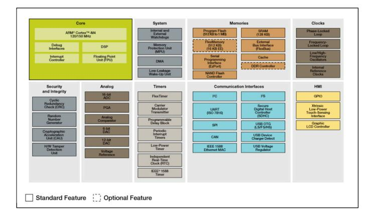
View additional information for Kinetis® K70-120–150 MHz, High-Speed USB, Ethernet, DDR and Anti-Tamper Microcontrollers Based on Arm® Cortex®-M4 Core.
