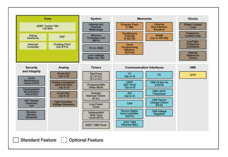
View additional information for Kinetis® K63-120 MHz, 256KB SRAM, Anti-Tamper Microcontrollers (MCUs) based on Arm® Cortex®-M4 Core.
