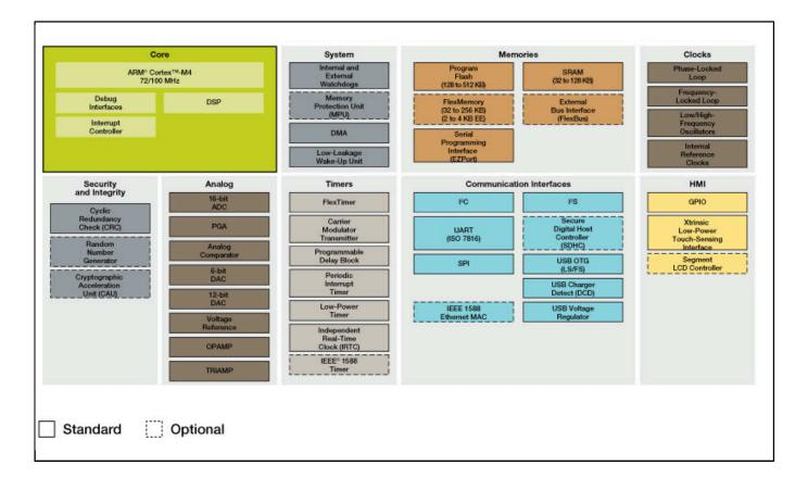
View additional information for Kinetis® K50-72 MHz, USB Microcontrollers (MCUs) based on Arm® Cortex®-M4 Core.
