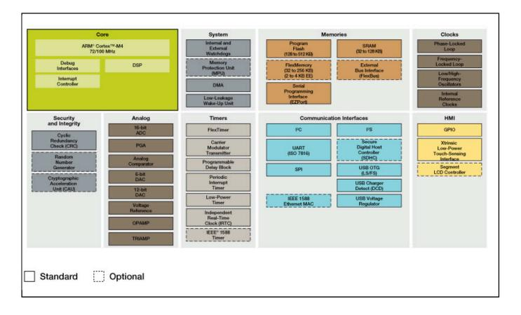
View additional information for Kinetis® K50-100 MHz, USB Microcontrollers (MCUs) based on Arm® Cortex®-M4 Core.
