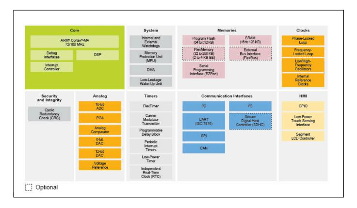
View additional information for Kinetis® K30-100 MHz, Mixed-Signal Integration Microcontrollers (MCUs) based on Arm® Cortex®-M4 Core.
