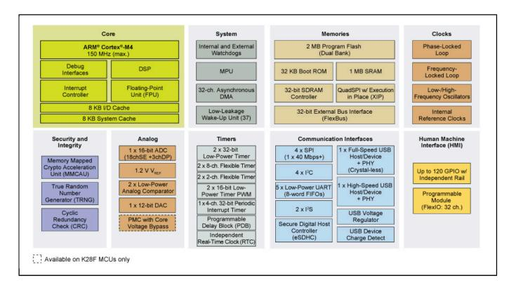
View additional information for Kinetis® K28-150 MHz, 2x USB, Core Voltage Bypass, 2MB Flash, 1MB SRAM MCUs based on Arm® Cortex®-M4.
