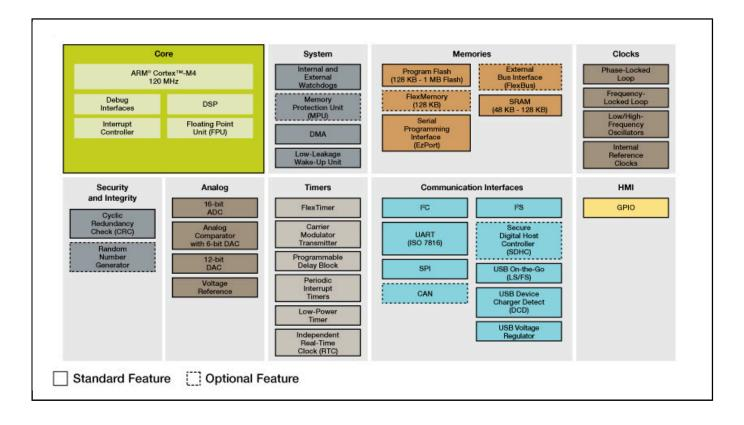
View additional information for Kinetis® K22-100 MHz, Cost Effective, Full-Speed USB Microcontrollers (MCUs) based on Arm® Cortex®-M4 Core.
