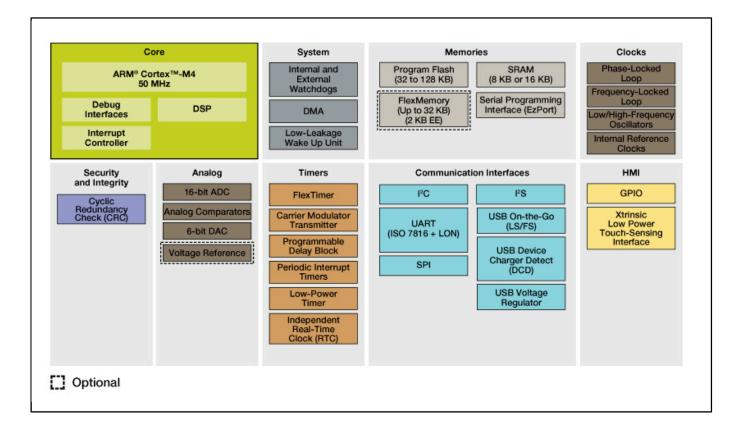
View additional information for Kinetis® K20-50 MHz, Full-Speed USB, Mixed-Signal Integration Microcontrollers based on Arm® Cortex®-M4 Core.
