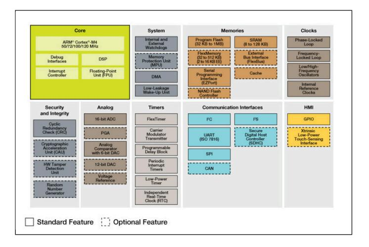
View additional information for Kinetis® K10-100 MHz, Mixed-Signal Integration Microcontrollers (MCUs) based on Arm® Cortex®-M4 Core.
