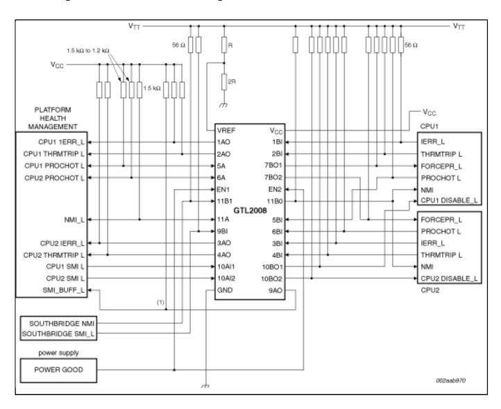
View additional information for 12-Bit GTL-to-LVTTL Translator with Power Good Control and High-Impedance LVTTL and GTL Outputs.
