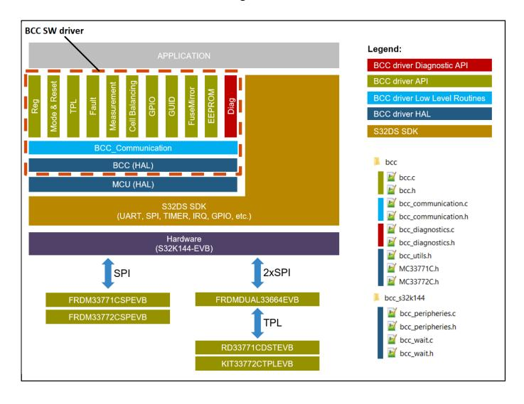
View additional information for Embedded SW: Battery Cell Controller Software Driver for MC33771C and MC33772C.
