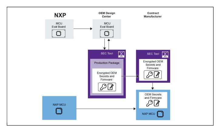
**Device HSM Trust Provisioning Flow Block Diagram**
