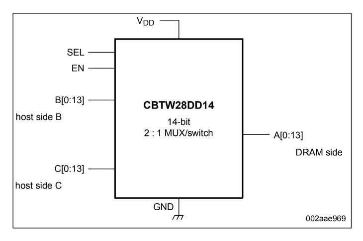
View additional information for 14-Bit Bus Switch/Multiplexer for DDR2/DDR3/DDR4 Applications.
