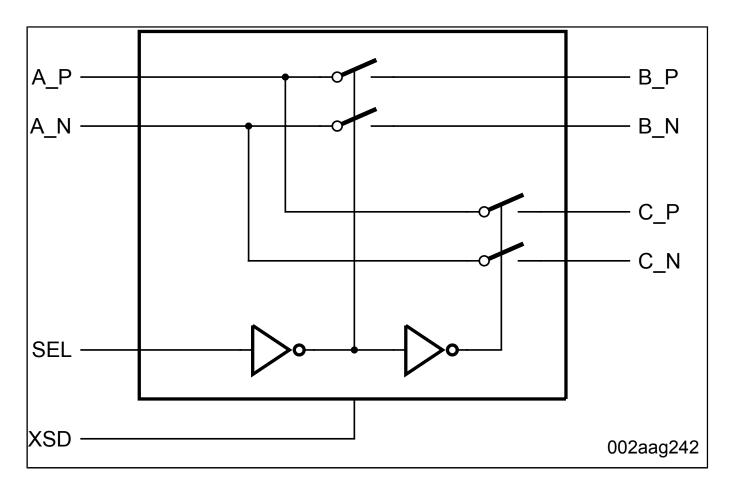
View additional information for 3.3 V, One Differential Channel, 2-1 Multiplexer/Demultiplexer Switch for PCI Express® Gen3.
