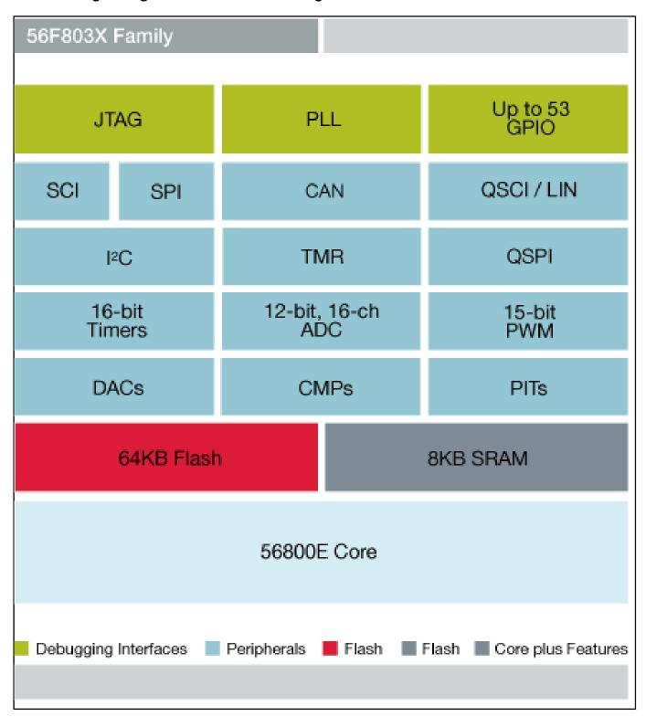
View additional information for Digital Signal Controller with CAN for Industrial Applications.
